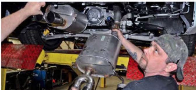
13 With the valves disconnected, the exhaust system should wiggle free of the factory crossover pipe, one side at a time.
